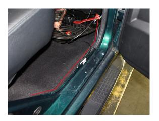
Eagle1 Lock wiring Vehicle Loom
