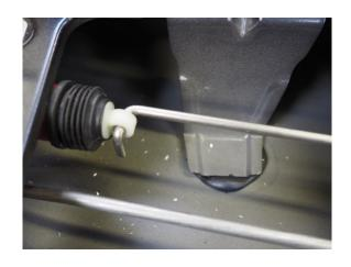
5) Remove the Factory fitting Key Lock rod from the Vehicle
