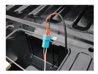
9) Connect cable using the scotch locks (or solder) please ensure the cables get a good connection
